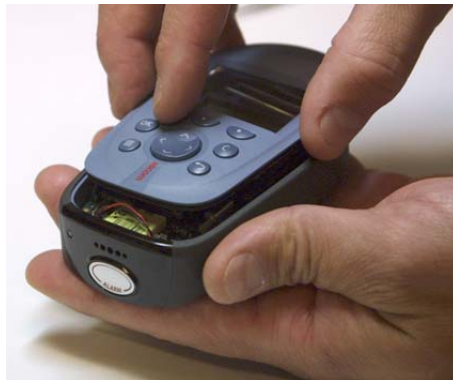
Figure 24. Closing the front. Be sure not to pinch the cable!
