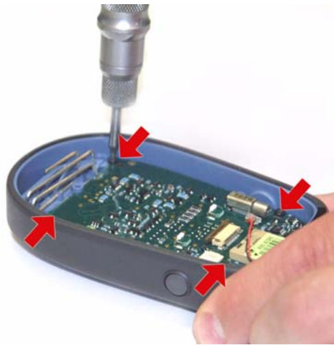
Figure 10. Releasing the four screws holding the circuit board
