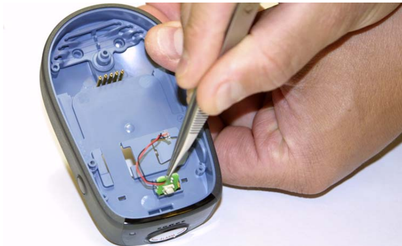
Figure 16. Inserting the push-button alarm contact
