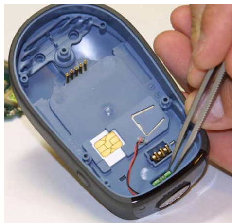
Figure 12. Lifting out the push-button alarm contact
